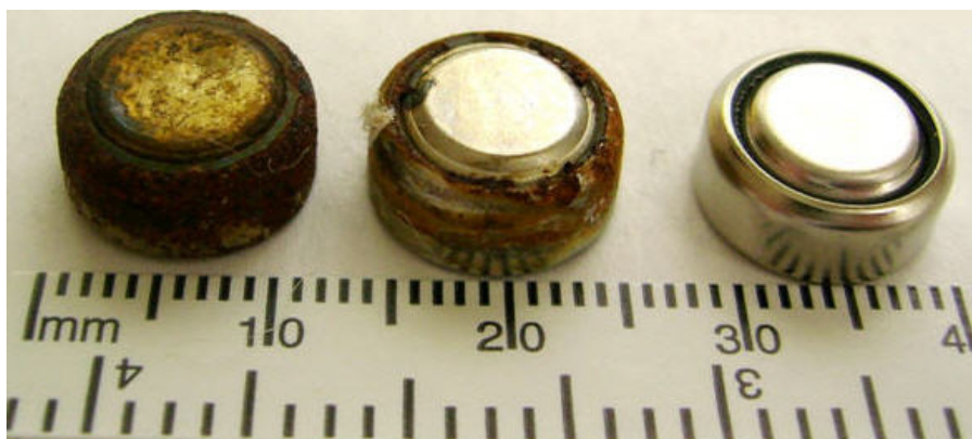
Figure 3. 1.5V batteries removed from Patients 3 and 4 as compared to a new battery (right side) of the same size. The battery on the left side (Patient 3) had been in the nose for 4 hours. The middle battery (Patient 4) was removed after approximately 1.5 hours; corrosion is already clearly visible on the casing
