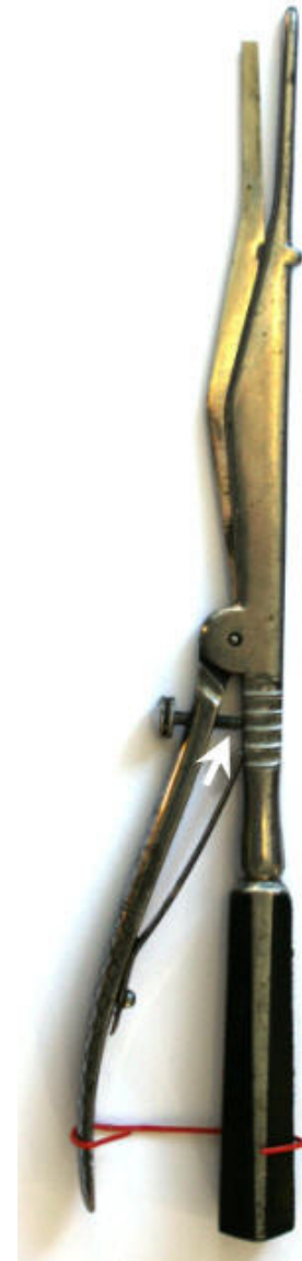
Figure 2. A screw (arrowed) limits the extent to which the knife (with its external cutting edge) can be opened
