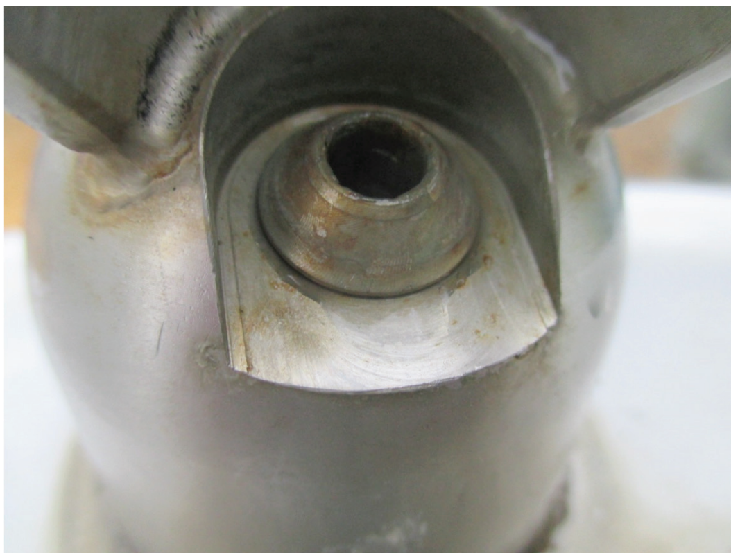
Figure 3: Example of discolouration (probably from biofilm) around a drinking fountain nozzle.
